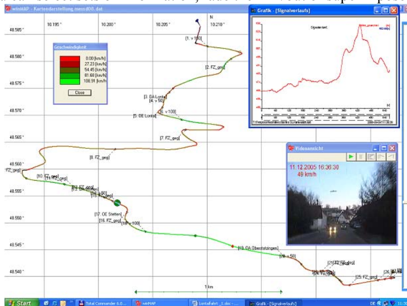
Figure 5 - Driving cycle: Recorded with winADAM and post-processed after analysing the video recording.
