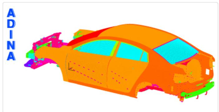
Automobile mesh consisting of continuum and structural elements
