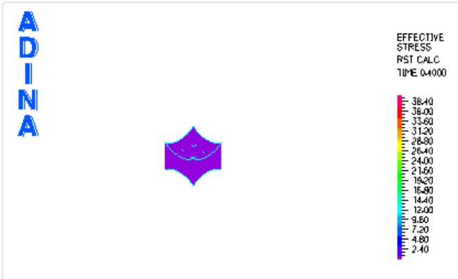
Stretching of a rubber component using the Mooney-Rivlin material model
