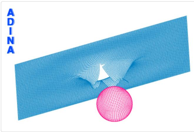
Steel ball impacting and punching through a thin plate
