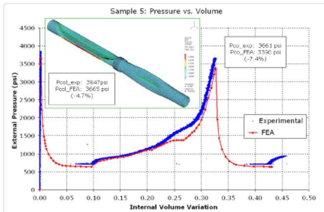
Collapse of Underwater Pipe
