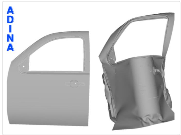
Crushing of an automobile door using self-contact analysis
