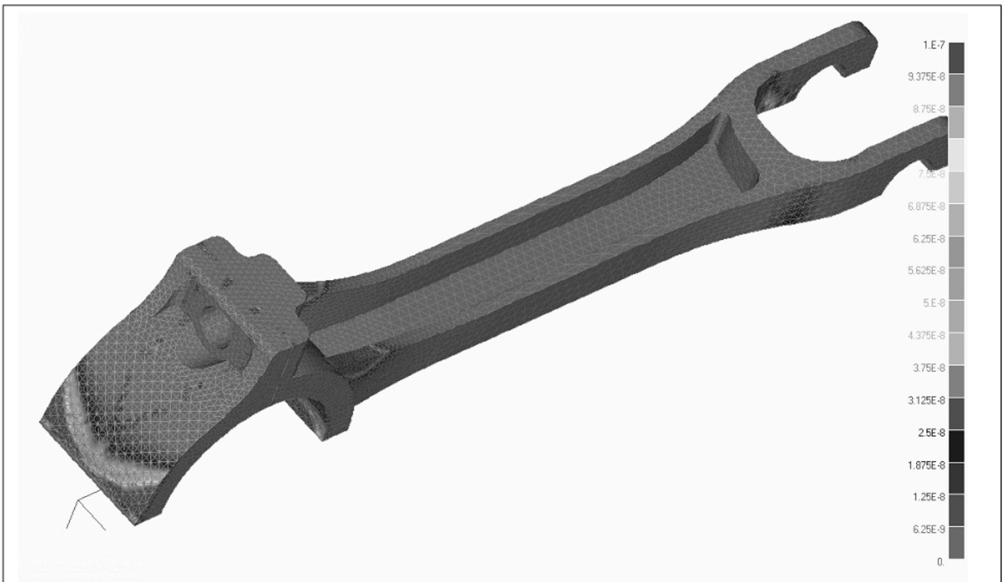
Fig. 30: result of fatigue calculation of the stabilisation beam of a heavy truck vehicle
